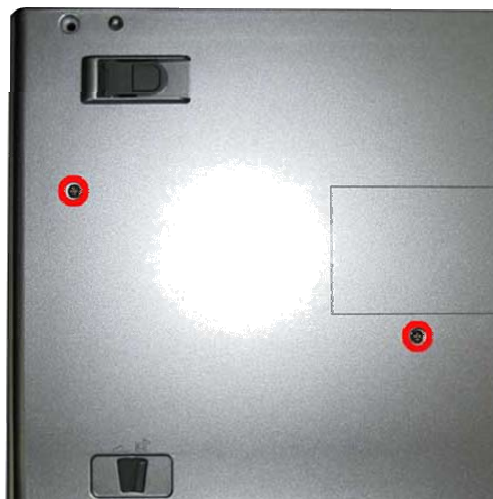
Fig. 10 Releasing the optical drive
